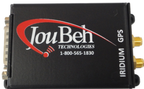
JouBeh 9602W SBD Satellite Transceiver Features RS-232 Serial Interface.
