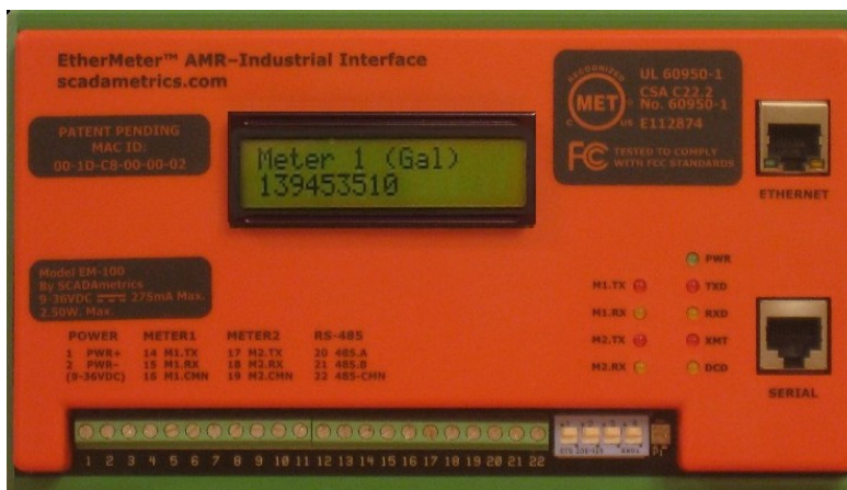
EtherMeter SCADA/Meter Gateway Equipped With Iridium Satellite Firmware.
