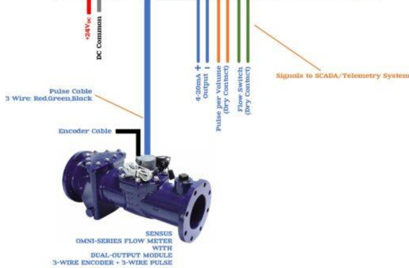
Example APK.PLUS Application: SCADA Analog Interface for Sensus Omni-Series Water Meter.
