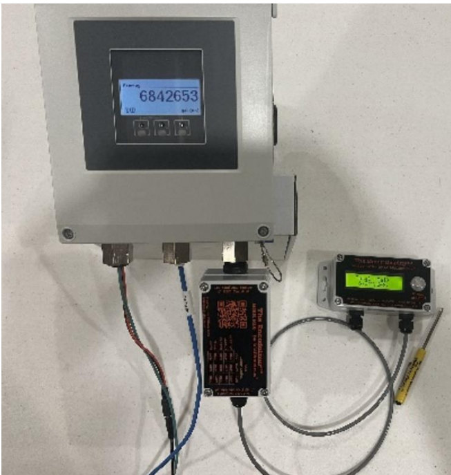
Endress+Hauser 1" Promag W 400 SCADAmetrics Model MBE Encodalizer™ SCADAmetrics Model TMD TheMeterDisplay™ - For Troubleshooting
