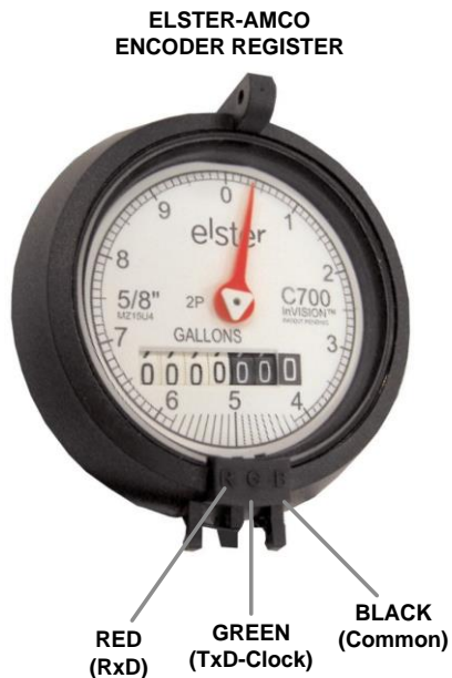
Figure 8A. Honeywell-Elster-AMCO InVISION – Register Diagram.
