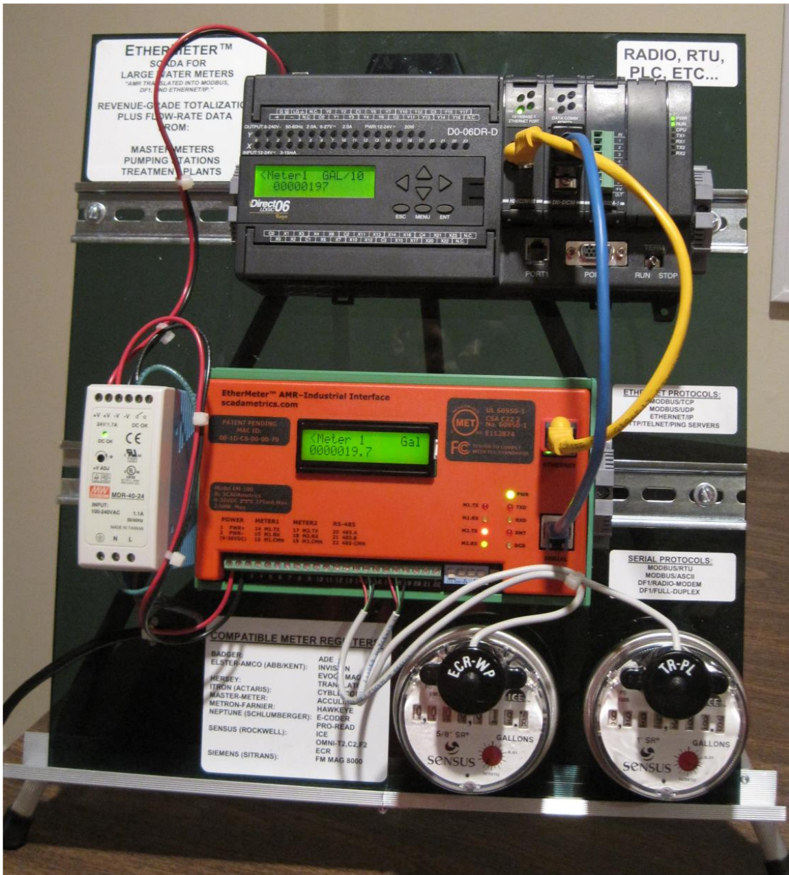
Figure 4. Koyo MODBUS Communication Demonstration Panel. DL06 PLC / EtherMeter Hardware and Wiring Configuration.
