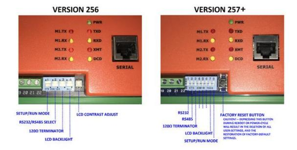
The **Version 256 EtherMeter** contained a 4-Position Dip Switch and a Contrast Adjustment Potentiometer for the LCD Display.
