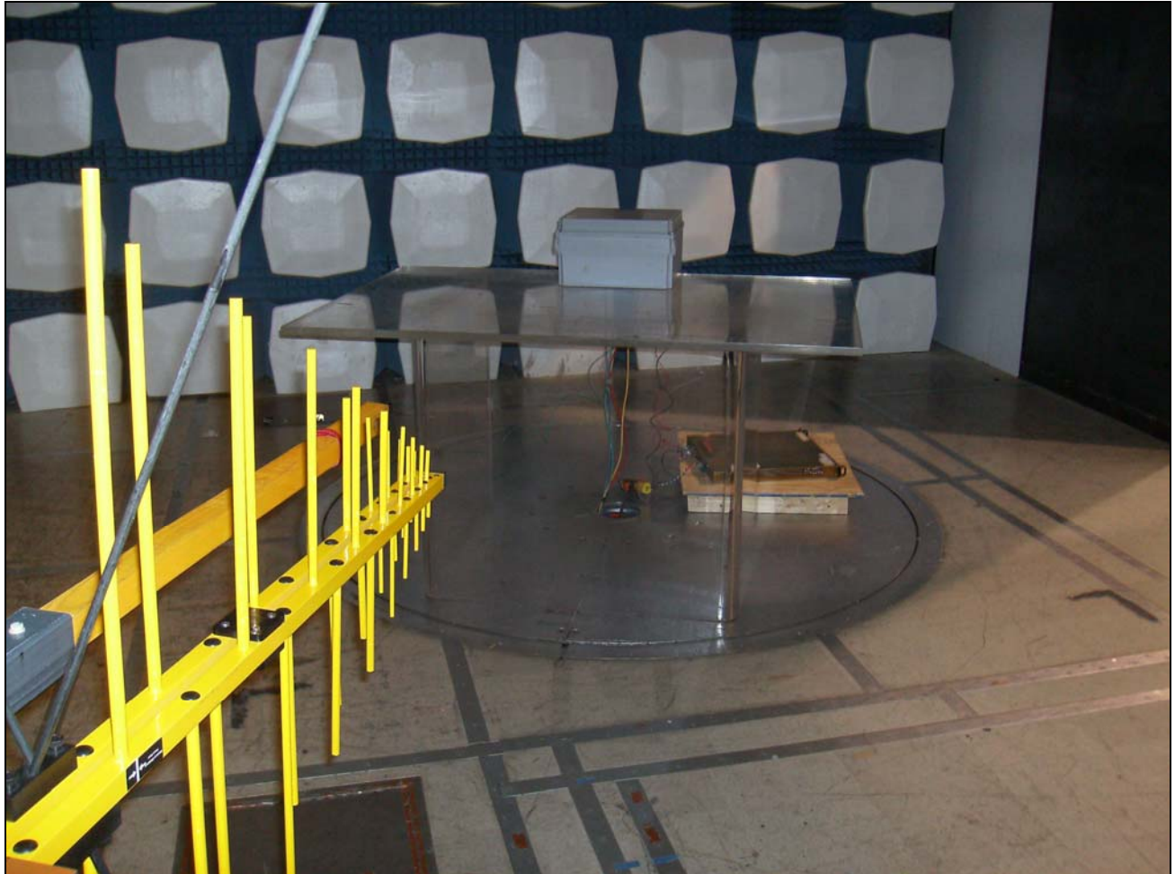
Photograph 1. Radiated Emission Limits Test Setup
