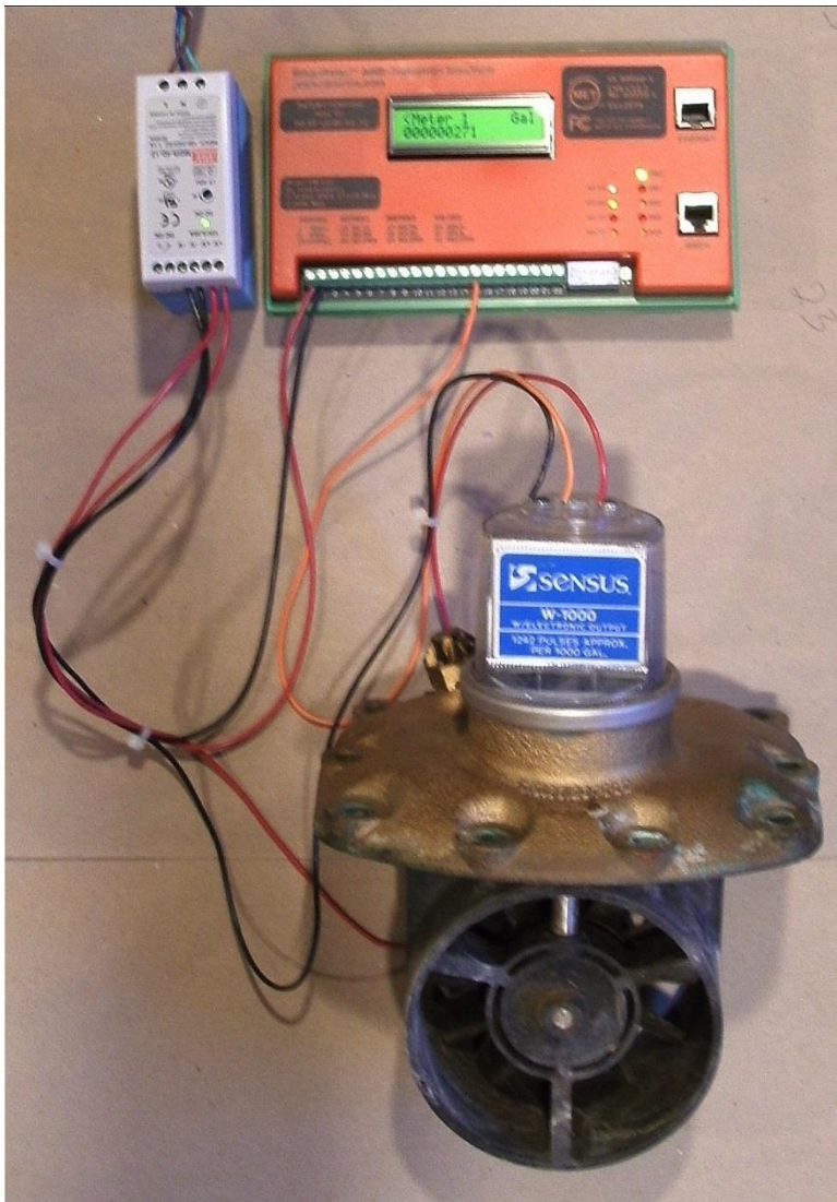
Figure 2. Sensus High-Speed Pickup / EtherMeter Laboratory Test Configuration. Powering The EtherMeter and High-Speed Pickup is a Meanwell MDR-40-12 (12VDC/40W Output).
