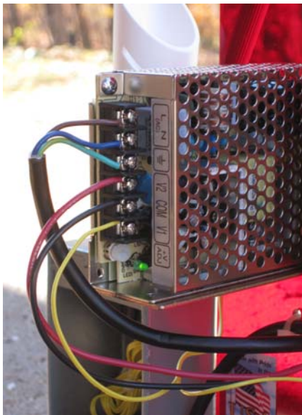
RD-35B Dual-Output Power Supply: 24VDC Powers The EtherMeter. 5VDC Powers The Thermistor.
