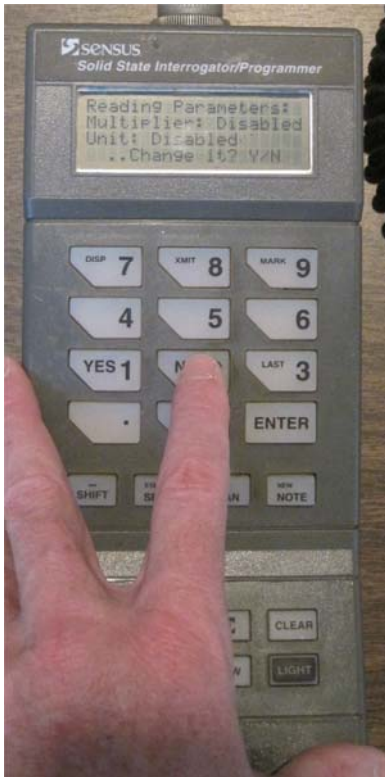
Figure 10. Reading Parameters: Multiplier: Disabled Unit: Disabled Change it? Press the “NO” key.
