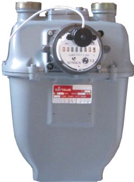
Figure 1. A Sensus R-175 Gas Meter Equipped With An Encoder-Based “ICE” Index (Register). This particular meter, when programmed to transmit all eight (8) digits, provides 1 cubic foot resolution and totalizes up to 99,999,999 cubic feet.
