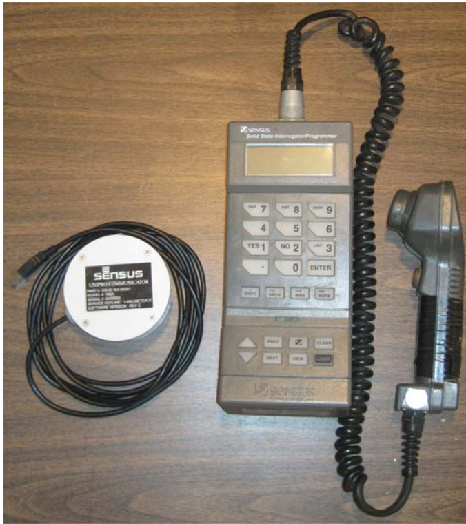
Figure 2. A new Sensus UniPro 100A Programmer (Left), and a legacy Sensus Model 3001 Programmer (Right).
