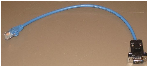
Figure 3. Completed EtherMeter-D0-DCM Cable.
