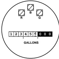
When using a meter register which transmit 6 digits of resolution, the totalization usually changes quite slowly for a properly-sized meter. In these instances, the least significant odometer wheel (the rightmost wheel) may be observed to be turning at a very slow RPM rate.
